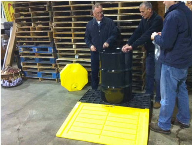
New spill containment pads installed
