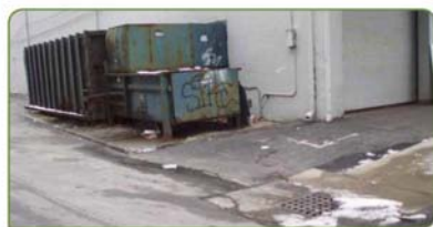
Examples of uncovered dumpsters with evidence of leakage and "dumpster juice" trails leading to nearby storm drain inlets.
